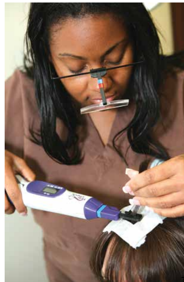
The HairCheck® tool can accurately determine the amount and quality of hair growing in a given area of the scalp to gauge the severity of hair loss and measure results during treatment
